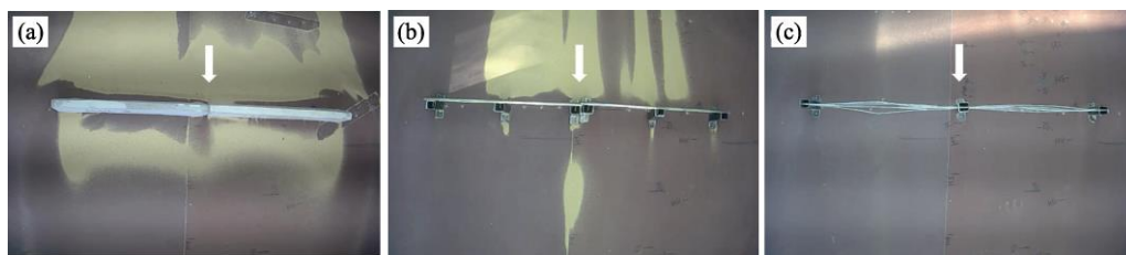
Fig. 12 Sand deposition around the guardrail. (a), concrete guardrail; (b), W-beam guardrail; (c), cable guardrail.
